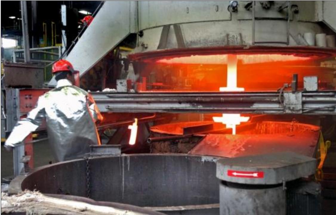
A worker in a production area at Rex Heat Treat in Lansdale removes a metal part following a quenching procedure.
