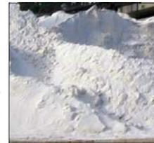
Quartz sand (silica) is the main raw material in commercial glass production.
